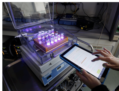
Figure 9. New design of the photoreactor with Bluetooth interphase.
